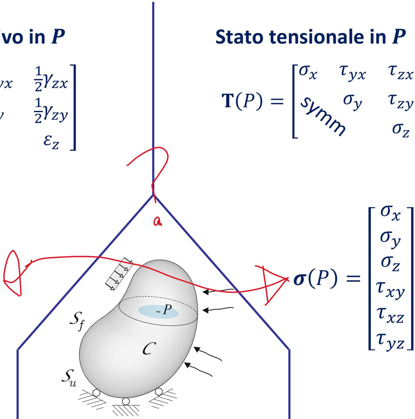
$$\boldsymbol{\sigma}(P) = \begin{bmatrix} \sigma_x \\ \sigma_y \\ \sigma_z \\ \tau_{xy} \\ \tau_{xz} \\ \tau_{yz} \end{bmatrix}$$
